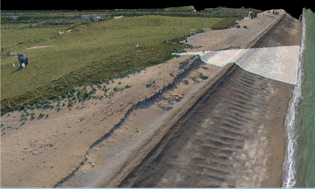
Figure 5: Fixed-wing and rotary RPA surveys at Sizewell (top left) and Hinkley Point (top right), and a Cefas RPA photo-topographic model of Cley Beach (Norfolk) viewed in perspective and illustrating the extraction of a beach profile, Norfolk (bottom).
